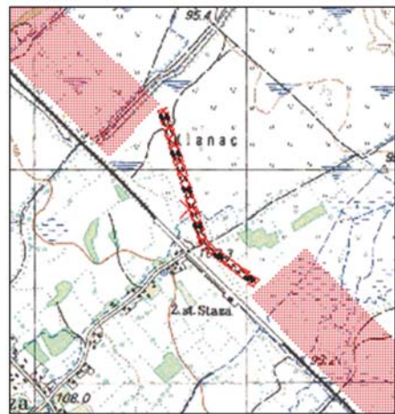
Reconstruction of MEO polygon according to the record with assesment of obstacles belt in front of the railroad
