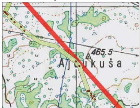
Demining results: found mines correlate to type but are outside of MEO reconstruction- pic.2.5.1
