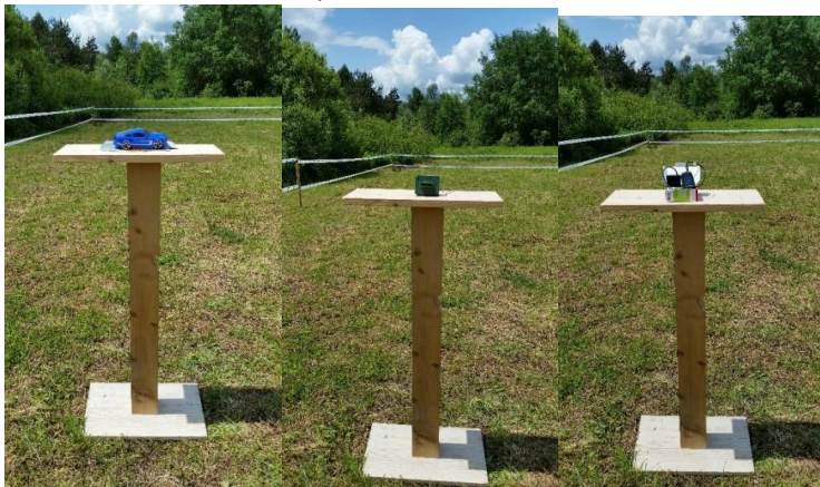
Figure 4.1 Toy car, IR sensor, NOKIA1616+El Switch at 1.20 m.
