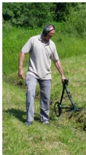
Figure 4.22: Following the signal of the wire positioned on the bottom of a ditch covered with water
