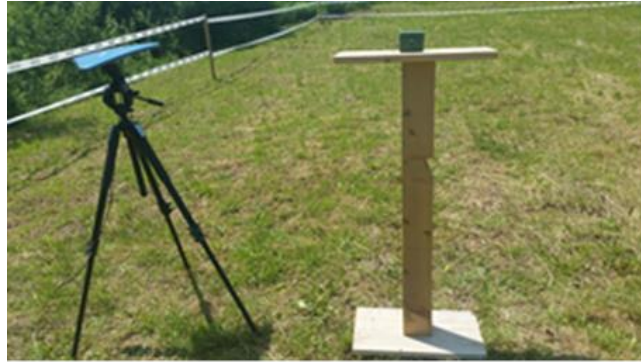
Figure 3.7: a) The spectrum of NR-900EK3M EAGLE transmitter was measured. b) by Rohde Schwarz Spectrum Analyser FSH8.
