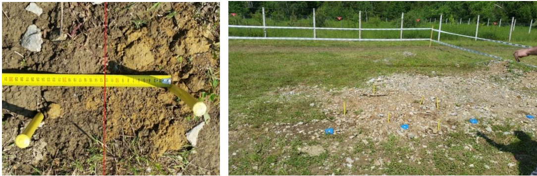
Figure 4.21: Boundaries of detection. c) Boundaries of wire detection with indicated (red line) wire orientation. b) Boundaries of welded grid detection
