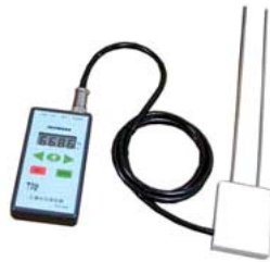
Figure 10. Time Domain Reflectometry (TDR) meter for volumetric water content measurement.
